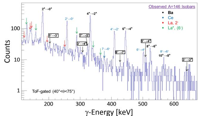
FIG. 2. The coincident  $\gamma$ -ray spectrum obtained by gating on the  $A = 146$  group in the CHICO2 TOF spectrum (Fig. 1). Many  $^{146}\text{Ba}$  transitions are seen along with lines from the radioactive isobaric contaminants that were also produced in CARIBU.
