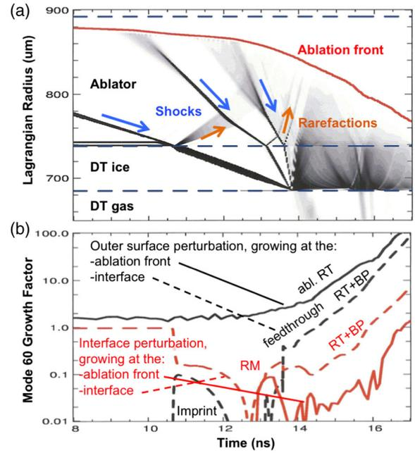
FIG. 2. (a) Shock trajectories, produced by plotting the logarithmic derivative of the pressure, plotted in Lagrangian coordinates. Shocks are timed to merge near the DT ice-gas boundary. (b) The feedthrough between the ablation front and fuel-ablator interface is shown through growth factors (normalized amplitudes) from a mode 60 outersurface perturbation (black) and an interface perturbation (red) growing at the ablation front (solid) or the interface (dashed).
