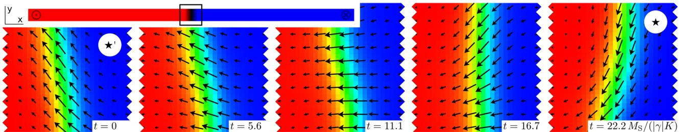
FIG. 4. Evolution of the magnetization during switching of DW chirality by means of an applied field  $H_z$  perpendicular to the film in a two-dimensional micromagnetic simulation. Only a part of the waveguide is shown. The arrows represent the direction of the in-plane component of magnetization  $\mathbf{m}(t, x, y)$  and the color the  $z$  component. We take  $H_z = 0.09K/M_S$ ,  $\alpha = 0.2$ ; other parameters are as in Fig. 3(b).
