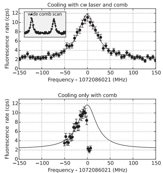
FIG. 3. Scan over line with and without additional cooling. The line in the lower plot is the fit to the spectroscopy data and is shown as a visual aid.
