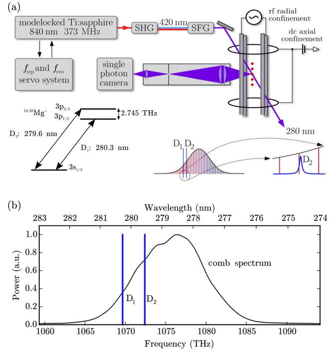
FIG. 1. (a) Schematic of the experimental setup. SPC: single photon camera, SHG: second-harmonic generation stage, SFG: sum-frequency generation stage and the comb spectrum after tripling into the UV. Blue lines,  $D_1$  and  $D_2$  lines of  $\text{Mg}^+$ . (b) Recorded comb spectrum. Vertical lines,  $D_1$  and  $D_2$  lines of  $\text{Mg}^+$ . Note that the envelope of the comb's spectrum is significantly blue detuned from both transitions.
