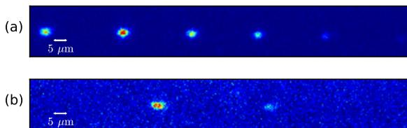
FIG. 2. (a) Image of a pure  $^{26}\text{Mg}^+$  ion crystal integrated during 300 s exposure while illuminated only with the frequency comb. The ions remain clearly crystallized for the entire time. (b) Two  $^{25}\text{Mg}^+$  ions cooled by the frequency comb. The scale bars on the images are  $5\ \mu\text{m}$  long.
