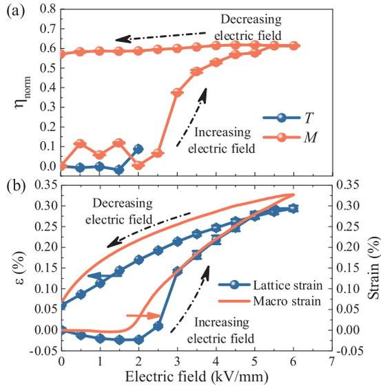
FIG. 3. (a) The influence of electric field on normalized relative domain fraction  $\eta_{\text{norm}}$  of the monoclinic and tetragonal phases. (b) Relative lattice strain of  $(200)_{\text{PC}}$  reflection  $\varepsilon$  of the monoclinic phase and the macrostrain measured by the ferroelectric analyzer for the PZT53.5 ceramic as a function of the electric field.
