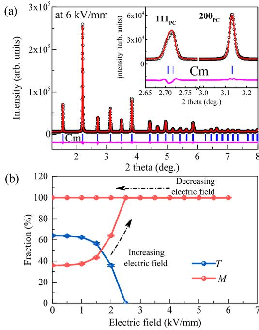
FIG. 2. (a) Structural refinement results of PZT53.5 at 6 kV/mm. The black asterisks indicate the raw diffraction data, red line corresponds to the calculated diffraction pattern, and the blue vertical ticks mark the calculated positions of  $Cm$  phase reflections. The insets show the enlarged profile of  $(111)_{PC}$  and  $(200)_{PC}$  reflections. (b) Phase fraction of the tetragonal and monoclinic phases as a function of the electric field. The error bars are smaller than the symbols.
