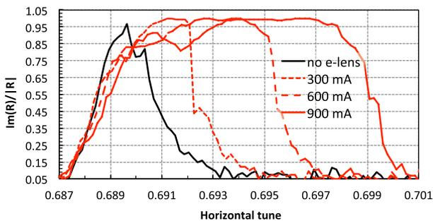
FIG. 4 (color online). Measured tune distribution as a function of the electron beam current without beam-beam collisions and with an electron beam size of  $\sigma_e = 0.55$  mm. The curves are aligned to the left with an offset for better visibility of the effect.
