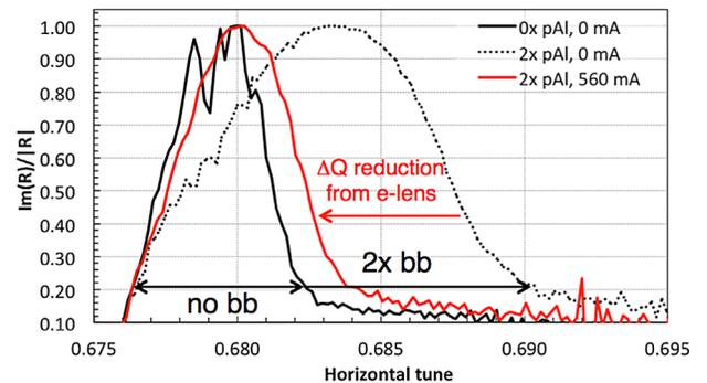
FIG. 5 (color online). Tune distribution width reduction with the electron lens, measured in the proton beam with  $p + \text{Al}$  collisions. The distribution widens due to two beam-beam interactions, and narrows again with the electron lens. The curves are aligned to the left with an offset for better visibility of the effect.
