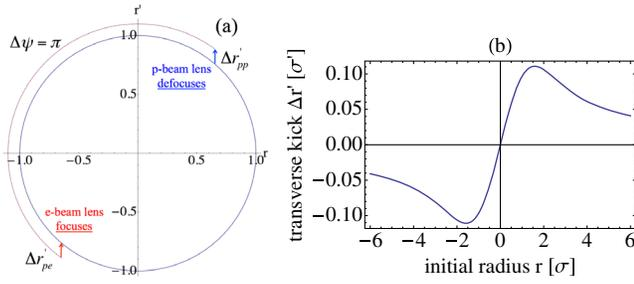
FIG. 1 (color online). (a) Head-on beam-beam compensation in a phase space view. A defocusing kick  $\Delta r'_{pp}$  that a proton receives from the other proton beam is reversed by a focusing kick  $\Delta r'_{pe}$  from the electron lens after a phase advance  $\pi$ . (b) Amplitude dependence of the beam-beam kick  $\Delta r'$  on the radius  $r$ .
