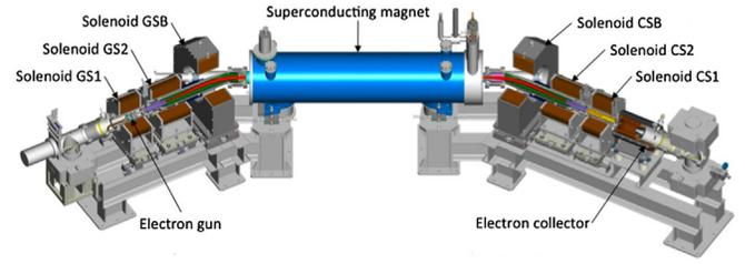
FIG. 2 (color online). One of two RHIC electron lenses. The electron beam moves from left to right and collides with the proton beam, moving from right to left, inside the superconducting solenoid.
