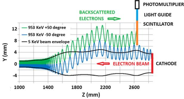
FIG. 3 (color online). Proton-electron beam overlap monitor. Electrons backscattered off protons are bent upwards in the gun solenoid bend (GSB) (see Fig. 2), pass through a 0.1 mm thin titanium alloy window, and are detected with a scintillator [20].
