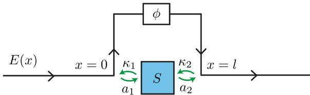
FIG. 1 (color online). Schematic of the setup. A unidirectional bosonic field,  $E(x)$ , interacts with the system,  $S$ , at positions  $x = 0$  and  $x = l$ . The interaction at  $x = 0$  ( $x = l$ ) is with a system operator  $a_1$  ( $a_2$ ) and a rate  $\kappa_1$  ( $\kappa_2$ ). We assume that an arbitrary phase shift,  $\phi$ , can be applied to the field between  $x = 0$  and  $x = l$ , such that the time delay,  $\tau = l/c$ , and the phase are independently controllable.
