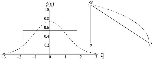
FIG. 1. Square (solid line) and Gaussian (dashed line) pointers of equal width  $\Delta = 1.5$  with (inset) the corresponding trade-off between the precision  $G$  and quality factor  $F$ .
