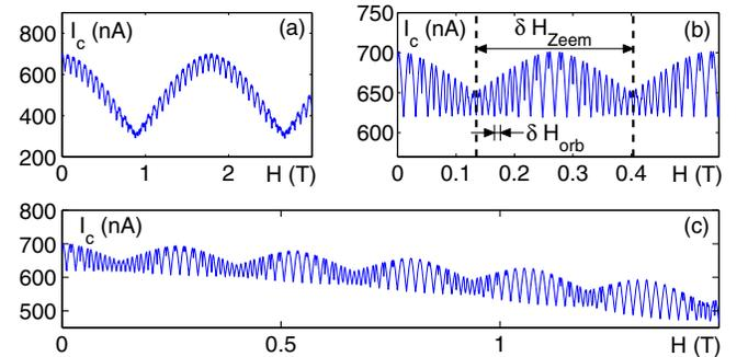
FIG. 2 (color online). The critical current  $I_c$  vs the magnetic field  $H$ . We choose  $T = 0.1$  K,  $\Delta_1 = 7.5$  K,  $\Delta_2 = 1$  K,  $v_F = 3 \times 10^5$  m/s,  $L = 2 \mu\text{m}$ , and (a)  $D = 15$  nm and (b), (c)  $D = 50$  nm. We also take (a)  $g_1 = g_2 = 1.5$ , (b)  $g_1 = 10$  and  $g_2 = 10$ , (c)  $g_1 = 1$  and  $g_2 = 10$ .
