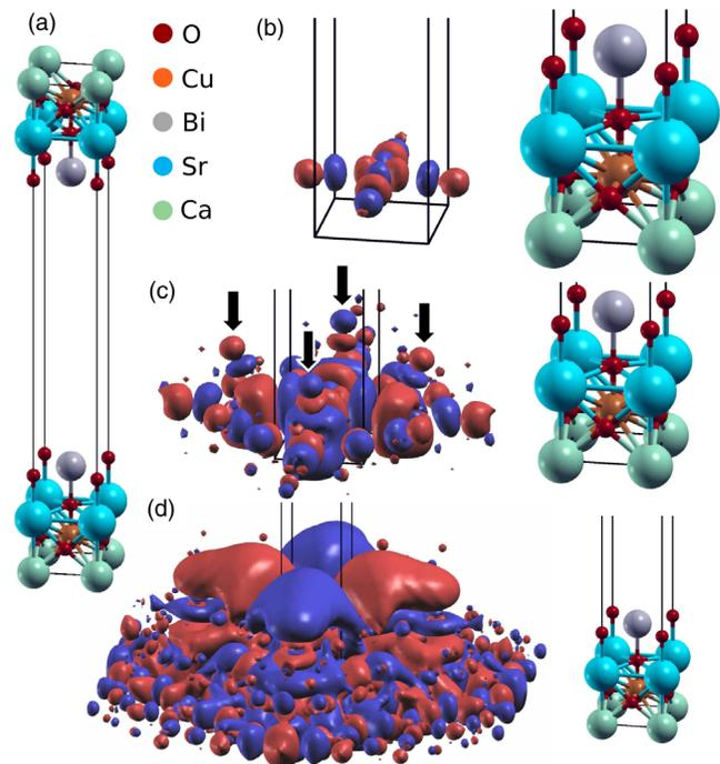
FIG. 2 (color online). (a) Elementary cell used in first principles calculation to obtain the electronic structure on the  $\text{Bi}_2\text{Sr}_2\text{CaCu}_2\text{O}_8$  surface. Isosurface plots of the Cu- $d_{x^2-y^2}$  Wannier function at (b) 0.05, (c) 0.005, and (d) 0.0002  $\text{bohr}^{-3/2}$ . Arrows indicate nearest-neighbor apical oxygen tails and red and blue indicate the sign of the Wannier function.
