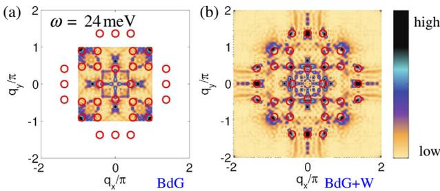
FIG. 4 (color online). Simulated QPI pattern from conductance maps: (a) Fourier transform of the lattice LDOS (BdG) and (b) Fourier transform of the continuum LDOS (BdG + W) at the same energy  $\omega = 24$  meV. Impurity potential for the weak scatterer  $V_{\text{imp}} = 0.3$  eV. The red open symbols indicate the expected positions of the spots from the octet model.
