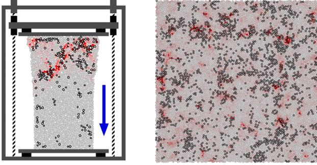
FIG. 1 (color online). Snapshot configurations of the two systems studied. Particles are colored gray to red according to their  $D_{\min}^2$  value. Particles identified as soft by the SVM are outlined in black. (a) A snapshot of the pillar system. Compression occurs in the direction indicated. (b) A snapshot of the  $d = 2$  sheared, thermal Lennard-Jones system.
