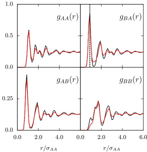
FIG. 3 (color online). Radial distribution functions averaged over hard (black dark lines) or soft (red light lines) particles.  $g_{AB}$  and  $g_{BA}$  functions of soft particles are not equal to each other since they refer to different kinds of regions: neighbors of soft particles from species  $A$  and neighbors of soft particles from species  $B$ , respectively.
