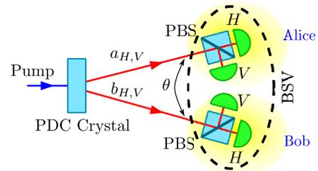
FIG. 1 (color online). Test of inequality (4) with four-mode squeezed vacuum state. Parametric down-conversion crystal (PDC) and polarizing beam splitter (PBS). The detectors measure photon numbers.
