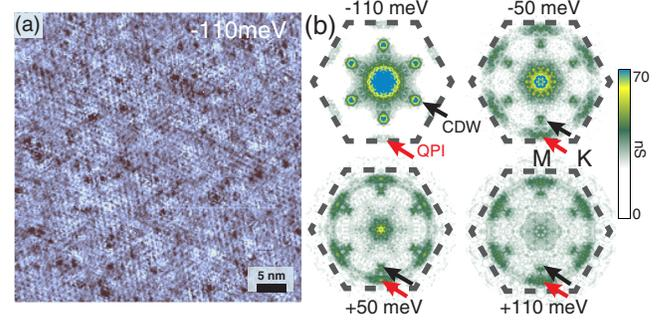
FIG. 2 (color online). (a) Real space  $dI/dV$  map at  $E = -110$  meV. The readily visible triangular lattice arises from the charge density wave (additional real space STS images shown in the Supplemental Material [14]). (b) Absolute value of the FFT of  $dI/dV$  maps at different energies showing nondispersing CDW peak (heavy arrow, black online) and QPI peaks dispersing with energy (light arrow, red online). Maps have been rotationally symmetrized as described in the main text.
