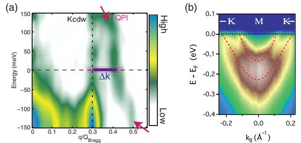
FIG. 3 (color online). (a) Line cut of the  $dI/dV$  maps in Fourier space along the  $\Gamma - M$  direction. The dashed line is a guide for the eye highlighting the position of the CDW ordering vector while the heavy line and shading (pink online) highlights the separation between the QPI intensity and the CDW wave vector at the Fermi energy. (b) ARPES (photon energy  $\approx 23$  eV) line cut along the  $K - M - K$  direction. The dotted line is the tight-binding fit to the data.
