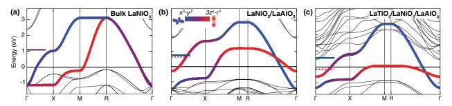
FIG. 1 (color online). Calculated  $1 \times 1$  band structures for (a) bulk LaNiO<sub>3</sub>, (b) two-component, and (c) three-component superlattices near the Fermi level with projections onto Wannier states represented by bold color shading. Horizontal lines indicate centers of  $3z^2 - r^2$  (red dashed) and  $x^2 - y^2$  (blue solid) bands.
