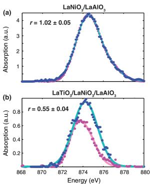
FIG. 3 (color online). Measured x-ray absorption (circles) for in-plane (blue) and out-of-plane (pink) polarizations of (a) twocomponent and (b) three-component nickelate superlattices. The solid colored lines are double Gaussian fits used in evaluating Eq. (1).
