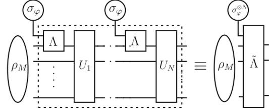
FIG. 2. Depiction of quantum channel simulation applied to the most general adaptive scheme (iv). It shows that, for a given simulation  $\Lambda$ ,  $\sigma_\varphi$ , the QFI of the scheme is bounded by  $F^{(iv)} = F[\Lambda(\rho_M \otimes \sigma_\varphi^{\otimes N})] \leq NF(\sigma_\varphi)$ .
