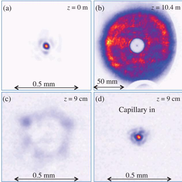
FIG. 1 (color). Typical laser spatial profiles in a vacuum with laser energy 16 J for (a) focus, (b)  $z = 10.4$  m downstream of focus, and (c)  $z = 9$  cm downstream of focus. The near field (b) shows an approximately top-hat profile. In (d) the guided mode is shown for plasma density  $7.5 \times 10^{17} \text{ cm}^{-3}$ . Well-confined high-quality modes were observed for densities as low as  $2 \times 10^{17} \text{ cm}^{-3}$ . The color scale is the same for (c) and (d).
