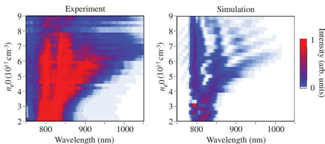
FIG. 3 (color). Measured (left panel) and simulated (right panel) optical spectra at the output of the 500- $\mu\text{m}$ -diam capillary as a function of plasma density for input laser energy  $\approx 7.5 \text{ J}$  and pulse duration  $\approx 40 \text{ fs}$ . The spectral response of the detection system was applied to the simulated data.
