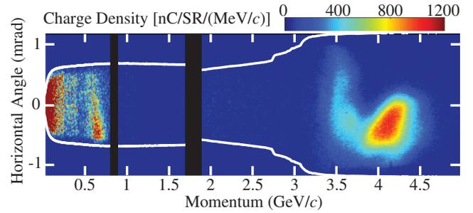
FIG. 5 (color). Energy spectrum of a 4.2 GeV electron beam measured using the broadband magnetic spectrometer. The plasma conditions closely match those in Fig. 2(c). The white lines show the angular acceptance of the spectrometer. The two black vertical stripes are areas not covered by the phosphor screen.
