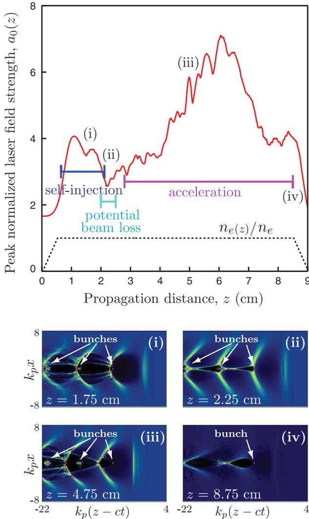
FIG. 4 (color). Evolution (a) of the peak normalized laser field strength,  $a_0(z)$  (red plot), in a PIC simulation for a top-hat laser pulse with an energy of 16 J focused at the entrance of a 9-cm-long plasma channel. The on-axis density (black dashed line) has a plateau density of  $n_e = 7 \times 10^{17} \text{ cm}^{-3}$ , and the matched radius is  $r_m = 81 \mu\text{m}$ . The wakefield (electron density) at various longitudinal locations is shown in (i)–(iv).
