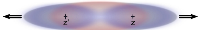
FIG. 1 (color online). Schematic of an axially freely expanding quasi-1D gas in a fragmented condensate many-body state. The two macroscopically occupied orbitals are indicated by red and blue shaded areas. Density correlations are measured at two (opposite) points z and z' in the cloud at some given instant t .
