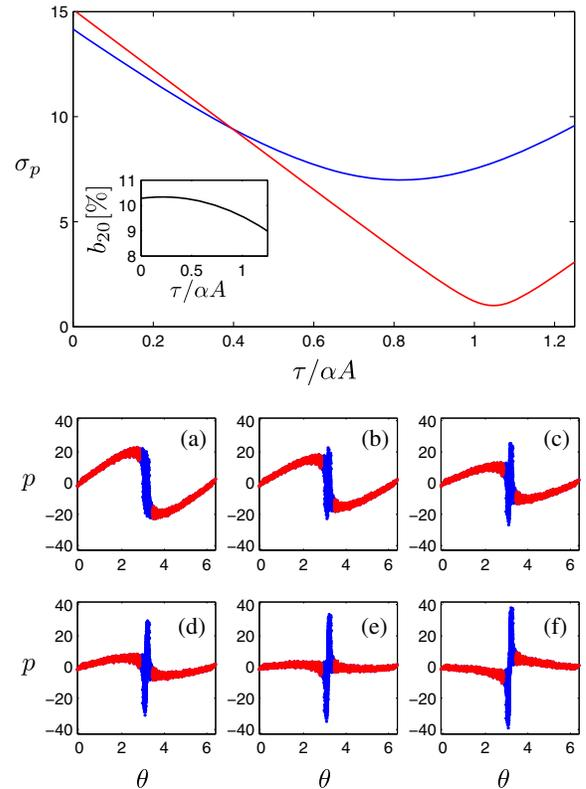
FIG. 2 (color online). Top: Evolution of the relative energy spread for the whole beam (blue) and the WP just outside the density spike (red). Inset: Evolution of the bunching factor for the 20th harmonic. Bottom: Phase space evolution along the drift.
