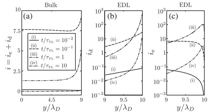
FIG. 4. Axial current densities computed for  $\Delta\phi = 7.5\phi_{th}$  in the middle of a single straight pore. (a) The total current in the bulk ( $0 < y/\lambda_D < 9$ ) rises and falls as the charging front passes. Within the EDL ( $9 < y/\lambda_D < 10$ ), the (b) diffusive and (c) Ohmic current densities also rise and fall, but are 2–3 orders of magnitude stronger, revealing the importance of surface conduction at high potentials.
