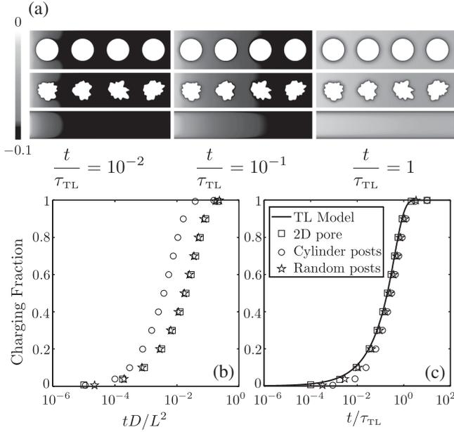
FIG. 2. The computed charging fraction [Eq. (7)] of three model electrodes at  $\Delta\phi = 0.1\phi_{th}$ . (a) The potential front at three different times looks remarkably similar for three different electrode morphologies. (b) Naively scaling time yields an apparent dependence on electrode morphology. (c) Scaling time by the TL time scale [Eq. (4)] collapses all results onto the TL curve, confirming its validity at low potentials.
