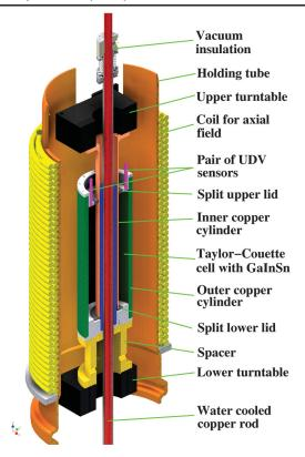
FIG. 1 (color). Sketch of the experimental setup.
