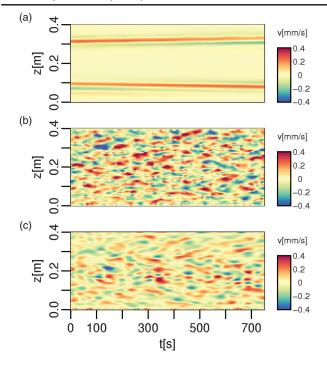
FIG. 2 (color). Velocity perturbation  $v_z(m=1,z,t)$  for  $\mu=0.26$ , Re = 1480, and Ha = 77. (a) 3D simulation for ideal axisymmetric field. (b) 3D simulation for realistic field. (c) Experimental results.
