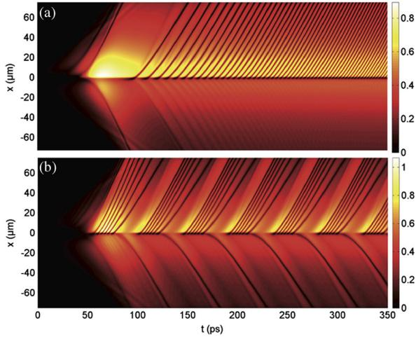
FIG. 3 (color online). Electric control of the dark soliton trains. (a) The potential step amplitude  $U(t)$  is linearly ramped down versus time from 0 to  $-1.5$  meV. (b) Sinusoidal modulation of the step between 0 and  $-1.5$  meV with a period of 50 ps.
