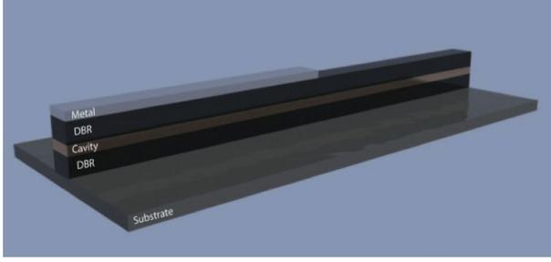
FIG. 1 (color online). Model of a potential sample consisting in a quasi-1D microcavity [distributed Bragg reflectors (DBR)] embedding a metallic deposition over half of its length to form a potential step. A gate voltage can be applied to the metal to tune dynamically the step amplitude.
