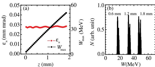
FIG. 3 (color online). (a) The normalized transverse emittance  $\epsilon_n$ , and the maximum energy  $W_{\text{max}}$  of the trapped electron beam versus acceleration distance  $z$ . (b) Electron beam energy spectra at  $z = 0.6 \text{ mm}$ ,  $1.2 \text{ mm}$ , and  $1.8 \text{ mm}$ . The laser-plasma parameters are the same as in Fig. 2.
