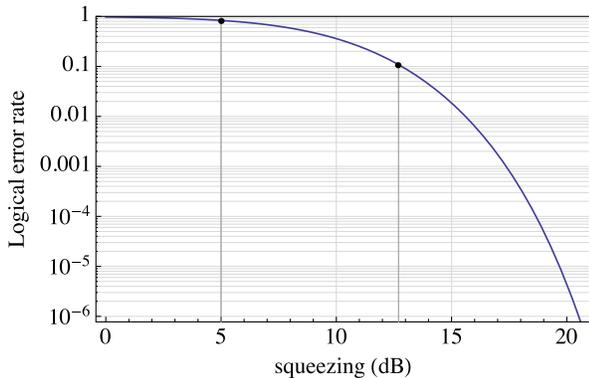
FIG. 1 (color online). Qubit-level logical error rate induced by GKP error correction with CV cluster states. The indicated level of squeezing is assumed to apply both to the initial momentum-squeezed states used to create the cluster state and in the Gaussian spikes that comprise the encoded GKP states. Also shown: maximum single-mode squeezing achieved to date (12.7 dB) [48,49] and squeezing achieved in a large CV cluster state (5 dB) [9].
