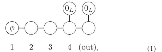
To implement gate  $\hat{G}$ , we must perform quadrature measurements associated with  $\mathbf{m}^{(G)}$  on nodes 1–4 on the bottom row. Measuring the ancillas (and appropriately displacing the nodes below) performs the GKP error correction on both  $\hat{q}$  and  $\hat{p}$ , as shown in Sec. I.A of the Supplemental Material [54]. To apply gates sequentially, one identifies the output node with node 1 of the next cluster.
