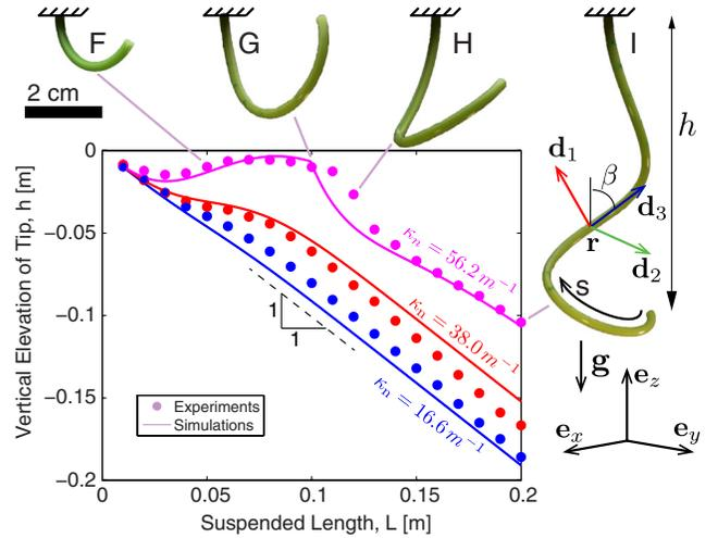
FIG. 2 (color online). Vertical elevation of the tip  $h$  versus arc length of the rod  $L$ , for three different natural curvatures  $\kappa_n = (16.6, 38.0, 56.2)$  m<sup>-1</sup>: experiments (circles) and simulations (solid lines). For  $\kappa_n = 56.2$  m<sup>-1</sup>, the configurations *F* and *G* are planar while the configurations *H* and *I* are nonplanar.
