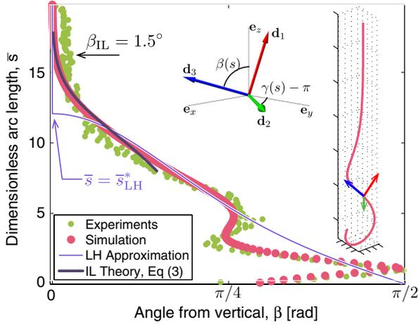
FIG. 4 (color online). A localized helical configuration as quantified by the angle from vertical,  $\beta(\bar{s})$ , for  $\bar{L} = 19.8$  and  $\bar{w} = 0.12$ . Experimental and numerical results are compared to the predictions from the local helix (LH) and inner layer (IL) approximations described in the text. The arrows show the predicted position of the transition point for each approximation.
