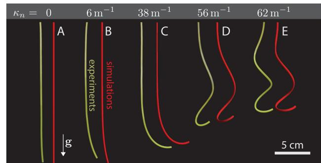
FIG. 1 (color online). Equilibrium shapes of rods suspended under their own weight: comparison of experiments and simulations. The natural curvature  $\kappa_n$  is varied, while the length  $L = 20 \text{ cm}$ , radius  $r = 1.55 \text{ mm}$ , elasticity parameters ( $E = 1290 \text{ kPa}$ ,  $\nu = 0.5$ ), and volumetric mass  $\rho = 1200 \text{ kg/m}^3$  are kept constant.
