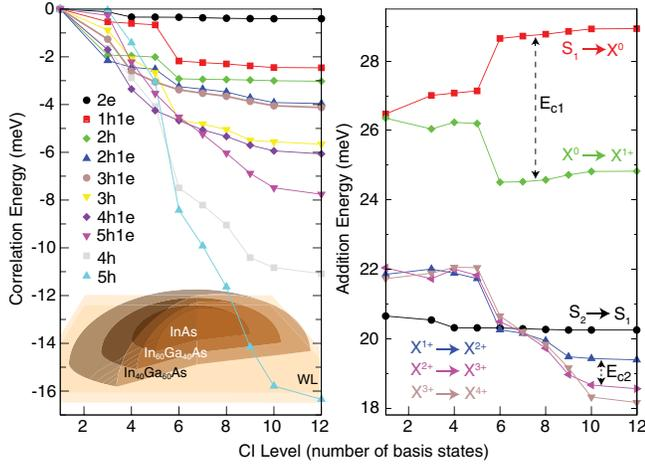
FIG. 4 (color online). Correlation (left) and addition (right) energies calculated with a varying number of basis states in a CI approach, for an InGaAs QD with a graded In composition (see inset in left panel). For five holes and one electron ( $5h1e$ ) using 12 basis states, the number of configurations amounts to 1,020,096, which is our present computational limitation.
