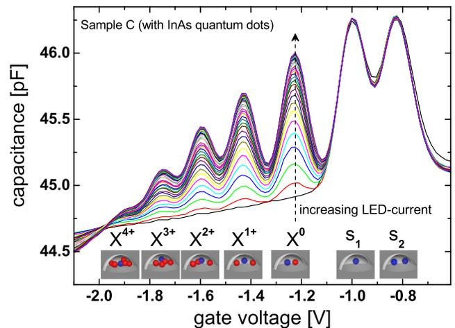
FIG. 2 (color online). Capacitance-voltage measurements under continuous illumination with various intensities on sample C (with QDs). We resolve five additional illumination-induced charging peaks, their occupancy by holes and electrons are indicated schematically by spheres.
