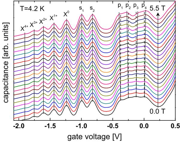
FIG. 3 (color online). Capacitance-voltage measurements under illumination ( $I = 72 \text{ W/m}^2$ ) with magnetic fields  $B$  ranging from 0 to 5.5 T (in steps of 0.5 T) perpendicular to the QD layer. Vertical dashed lines are guides to the eye.
