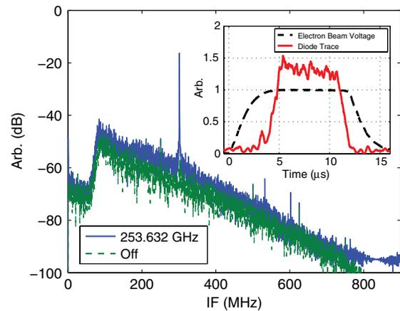
FIG. 4 (color online). Amplified pulse spectrum (blue) down-converted to  $f_{IF} = 300$  MHz. Also shown is the recorded noise spectrum (dashed green) during the voltage pulse when the rf driver is off. Insert: Diode trace measured at the gyrotron amplifier output and the corresponding high voltage pulse.
