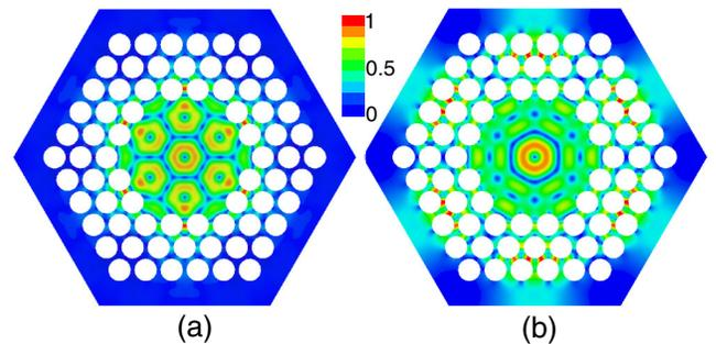
FIG. 2 (color online). Comparison between electric field of PBG waveguide modes with a cutoff frequency of (a) 242.7 GHz and (b) 212.1 GHz. The (a) operational  $TE_{03}$ -like mode is well confined ( $Q_{\text{diff}} = 1370$ ) and (b) the lower-order mode is not confined ( $Q_{\text{diff}} = 35$ ). The white circles are stainless steel rods with lattice constants of  $a = 0.397$  mm and  $a/b = 0.43$ .
