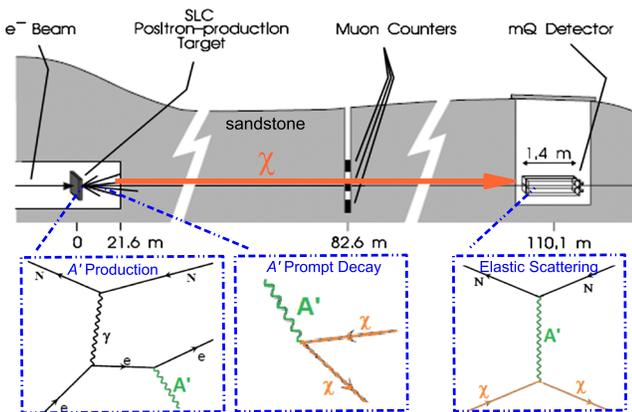
FIG. 1 (color online). Layout of the SLAC mQ experiment [11]. We investigate the possibility of  $A'$  production in the target, followed by prompt decay to long-lived dark-sector particles  $\chi$ , which could traverse the sandstone and undergo elastic scattering off carbon nuclei in the detector.
