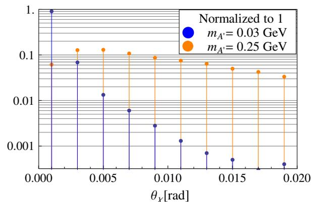
FIG. 2 (color online). Sample MG/ME  $\chi$  angular distributions ( $m_\chi = 10$  MeV). mQ angular acceptance is 0.002 rad.  $m_{A'} = 0.03$  GeV (steep curve) is 90% accepted.  $m_{A'} = 0.25$  GeV (shallow) is 6% accepted.
