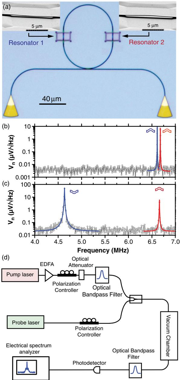
FIG. 1 (color online). (a) Micrograph of a racetrack cavity with two  $110 \text{ nm} \times 500 \text{ nm} \times 10 \text{ } \mu\text{m}$  suspended portions as nanomechanical resonators. Insets show scanning electron micrographs of the mechanical resonators in buckled down (left) and buckled up (right) state. (b), (c) thermal noise spectra in the up-up (b) down-up state (c). (d) The measurement setup with a weak probe laser, and a pump.
