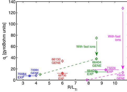
FIG. 5 (color online). Comparison of nonlinear GENE simulations and experimental ion heat flux measurements for the five separate discharges at  $\rho = 0.33$ . The importance of the fast ion contribution is underlined by the sensitivity studies carried out for discharges 66404 and 73224. The dashed lines connect the results of the nominal 66404 and 73224 simulations with results obtained at reduced  $R/L_{Ti}$ .
