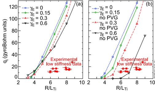
FIG. 2 (color online). Ion heat flux in nonlinear GENE  $R/L_{Ti}$  and  $\gamma_E$  scans based on discharge 70084 parameters at  $\rho = 0.33$  ( $q/\epsilon = 11.8$  for circular geometry).  $\hat{s}/q = 0.2/1.3$  throughout. Results are shown both including (a) and neglecting (b) PVG destabilization. All runs were electrostatic, collisionless, used circular geometry, and assumed  $T_e/T_i = 1$ . The results are compared with the low stiffness data from Ref. [7].
