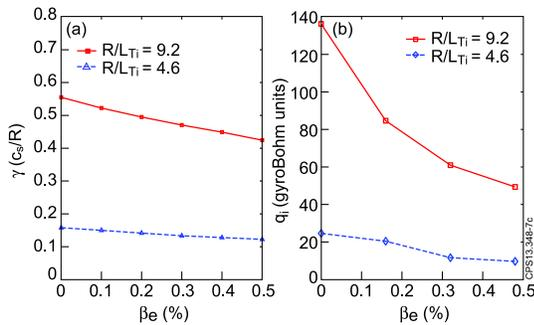
FIG. 3 (color online). Linear growth rates (a) and nonlinear ion heat fluxes (b) calculated in  $\beta_e$  and  $R/L_{Ti}$  scans based on discharge 66404 parameters. In the linear scan,  $k_y = 0.4$  in units of  $1/\rho_s$ . Runs included collisions, experimental geometry, two species, and assumed  $T_e/T_i = 1$ .
