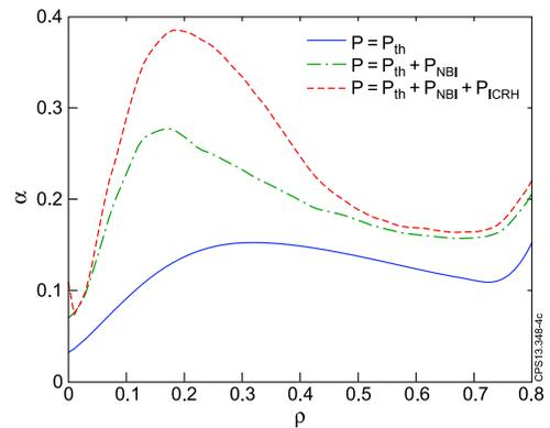
FIG. 4 (color online). The comparative influence of thermal and suprathreshold pressure components on  $\alpha$  for discharge 66404. Increased  $\alpha$  corresponds qualitatively to increased electromagnetic stabilization. The strong influence of suprathreshold pressure for  $\rho < 0.4$  coincides with the measured low stiffness zone.
