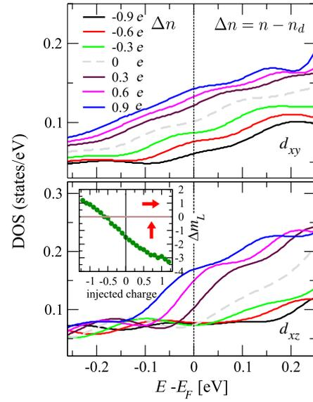
FIG. 3 (color online). Decomposed minority  $d$ -orbital local density of states (LDOS) for the Fe layer in the case of the system depicted in Fig. 1, for same representative charge-doping values,  $\Delta n = n - n_d$  where  $n(n_d)$  refers to the number of electrons in the charged (neutral) system, respectively. Inset: orbital moment differences ( $\Delta m_L = m_L^x - m_L^z$  in units of  $10^{-2} \mu_B$ ). Arrows indicate the direction of the highest orbital contribution.
