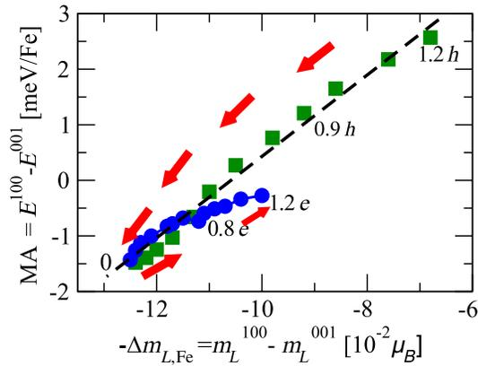
FIG. 4 (color online). Relationship between MA and OMA of the Fe bilayer in Pt/Fe<sub>2</sub>/Pt(100). Arrows indicate the direction of the MA behavior as a function of the injected electrons (holes).
