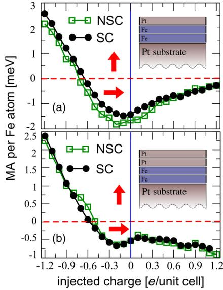
FIG. 2 (color online). Calculated self-consistent (SC) and non-self-consistent (NSC) MA per magnetic atom for (a) Pt/Fe<sub>2</sub>/Pt(100) and (b) Pt<sub>2</sub>/Fe<sub>2</sub>/Pt(100). The charge doping (in units of  $e$ /unit cell) has the same meaning than in Fig. 1. Positive (negative) MA values stand for an out (in-plane) axis of magnetization.
