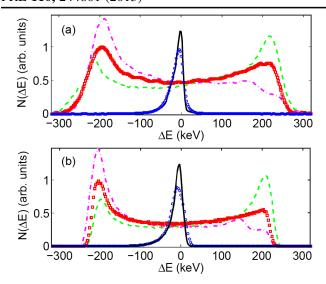
FIG. 4 (color online). Beam energy distributions in experiment (a) and simulation (b): with both lasers off (black solid lines); with only the first laser on (blue circles); with only the second laser on (red squares); net acceleration with both lasers on (green dashed lines); (e) net deceleration with both lasers on (magenta dashed-dotted lines).
