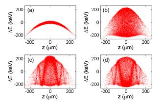
FIG. 5 (color online). Simulated beam longitudinal phase space at the entrance to (a) and exit of a cascaded IFEL [(b), (c), (d)]: (b) with only the second laser on; (c) net acceleration with both lasers on; (d) net deceleration with both lasers on.
