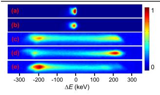
FIG. 3 (color online). Measured beam energy distribution: (a) with both lasers off; (b) with only the first laser on; (c) with only the second laser on; (d) net acceleration with both lasers on; (e) net deceleration with both lasers on. The beam intensity in (a) and (b) is reduced by a factor of 7 to avoid saturation using the same scaling as (c), (d), and (e).
