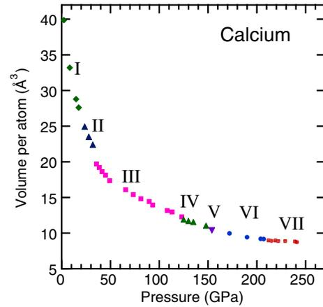
FIG. 3 (color online). Pressure dependence of the atomic volume for calcium. Data points for Ca-VII were obtained by the Rietveld analysis with the  $P4_2/ncm-128$  model. Numerical values for Ca-VII are given in Table S2 in the Supplemental Material [39].
