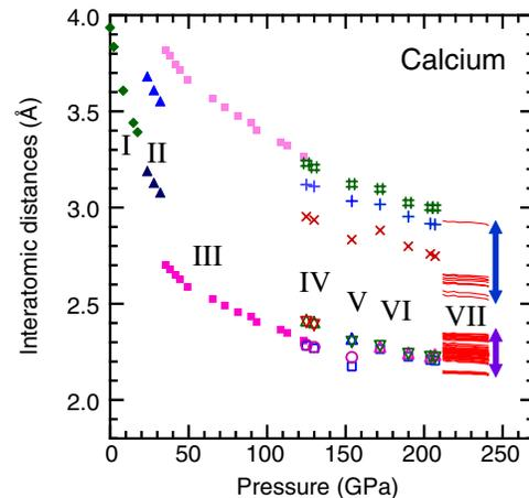
FIG. 4 (color online). Pressure change of the interatomic distances for calcium. Ca-VII data include numerous distances; therefore, its data points are marked with thin lines.
