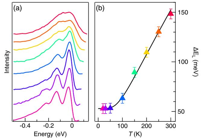
FIG. 3 (color online). (a) Spectra measured between  $T = 20$  K and  $T = 300$  K on a sample with  $n_e \approx 5 \times 10^{18} \text{ cm}^{-3}$ , showing a progressive broadening with increasing temperature. The signal extracted from the shallow electron pocket was integrated over a momentum range of  $-k_F < k_x < k_F$ . (b) Temperature-dependent intrinsic QP line width. Colors of the symbols correspond to those of the spectra in (a). The line is a Bloch-Grüneisen curve.
