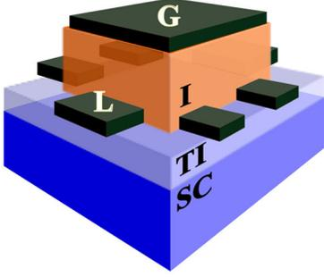
FIG. 1 (color online). The heterostructure device that can host fractional TR-invariant quantum states. A topological insulator (TI) quantum well is sandwiched between a conventional superconductor (SC) and a conventional insulator (I). The gate (G) voltage can be used to control the state of the TI, and the topological properties of the TI can be probed via a Hall-bar setup of leads (L).
