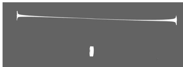
FIG. 1. Polyethylene sample before (bottom, diameter 9 mm) and after (top) stretching. The midplane deformation corresponds to a Hencky strain of 6.7. The Hencky strain in the filament midplane is measured on-line by a laser micrometer during the experiment.
