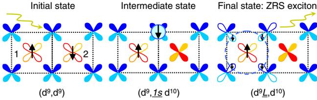
FIG. 2 (color online). Schematic illustration of how a ZRS exciton is created in the RIXS process at the oxygen  $K$  edge. See text for detailed explanations. Unoccupied states are depicted with empty orbitals.
