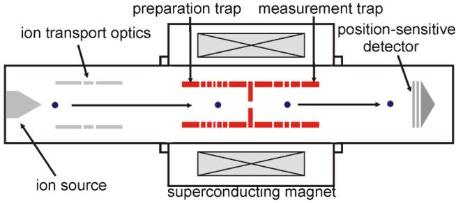
FIG. 1 (color online). Schematic of the setup used for the measurement of the mass difference between  $^{130}\text{Xe}$  and  $^{129}\text{Xe}$ .
