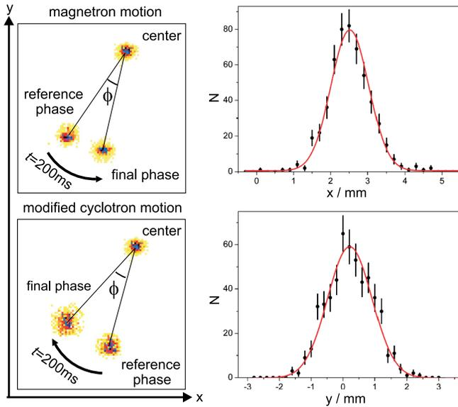
FIG. 4 (color online). (left-top) Magnetron and (left-bottom) modified-cyclotron projection figures of the  $\nu_c$  measurement of  $^{130}\text{Xe}^+$ . (right)  $N(x)$ , and  $N(y)$  projections of the final phase of the cyclotron motion. The phases were fitted with a Gaussian.
