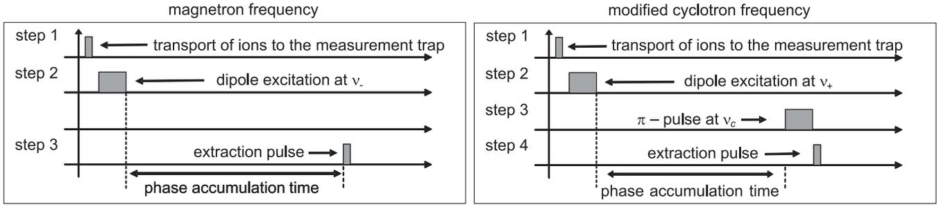
FIG. 3. Excitation pulse scheme for the measurement of the magnetron (left) and modified cyclotron (right) frequencies. For details see text.
