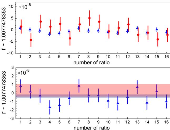
FIG. 5 (color online). Cyclotron-frequency ratios  $r$  of  $^{129}\text{Xe}^+$  to  $^{130}\text{Xe}^+$  measured in this work with the PI-ICR (blue triangles) and Ramsey TOF-ICR (red circles) techniques, respectively. The blue and red shaded bands are the uncertainties of the final ratios determined with the PI-ICR and Ramsey TOF-ICR method, respectively. The lower panel is a zoom of the upper panel.
