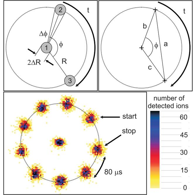
FIG. 2 (color online). Top: Principle of the measurement of the radial motions in a Penning trap (see text for details). Bottom: Experimentally recorded projection of the position of  $^{130}\text{Xe}^+$  ions for several phases of the magnetron motion with radius of approximately 0.5 mm in the measurement trap of SHIPTRAP.
