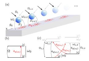
FIG. 1 (color online). Panel (a) Experimental scheme of the system: ensemble of equally spaced qubits placed in the vicinity of a one-dimensional waveguide. Panel (b) Two-level system configuration with resonant excitation. Panel (c): Four-level system configuration with two additional lasers, where we impose the condition:  $\omega_{L,1} - \omega_0 = \omega_{L,2} + \omega_0 = \omega_a$  and define  $\omega_1 = \omega_{L,1}, \omega_2 = \omega_{L,2} - \omega_0$ .
