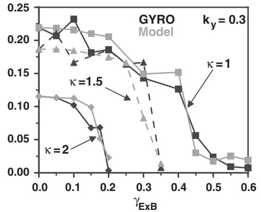
FIG. 3. Integrated intensity  $\bar{\Phi}_{ss}^2$  [Eq. (2)] at  $k_y = 0.3$  as a function of Doppler shear  $\gamma_{E \times B}$  for three values of the flux surface elongation ( $\kappa = 1.0, 1.5, 2.0$ ) comparing the GYRO results (black) with the spectral shift model (gray) [Eq. (7)].
