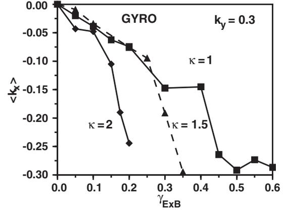
FIG. 2. The spectral average radial wave number shift [Eq. (2)]  $\langle k_x \rangle$  at  $k_y = 0.3$  as a function of the Doppler shear  $\gamma_{E \times B}$  computed from GYRO simulations for three values of the flux surface elongation ( $\kappa = 1.0, 1.5, 2.0$ ).
