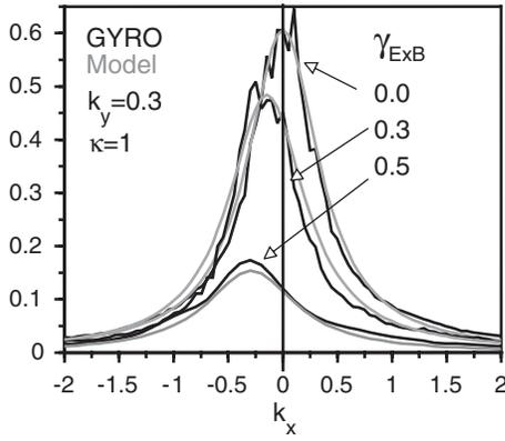
FIG. 1. Radial wave number spectrum of the time and flux surface averaged electric potential fluctuation Fourier amplitude  $\Phi_{k_y, k_x}$  (black) for the GA standard case [8] with  $k_y = 0.3$  and three values of the Doppler shear. Also shown are the spectral shift model spectra (gray) [Eq. (7)].
