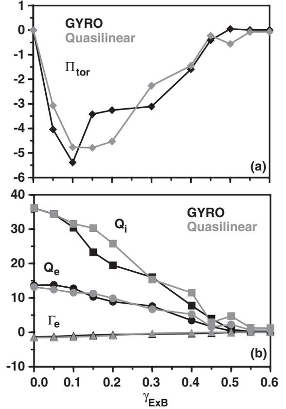
FIG. 4. Toroidal Reynolds stress (a) and electron and ion energy flux and particle flux (b) from GYRO simulations (black) and the spectral shift quasilinear model [Eq. (8)] (gray) as a function of Doppler shear rate for the GA standard case [8].
