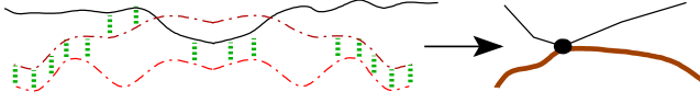
FIG. 1 (color online). Schematic diagram of strand exchange and the equivalent coarse-grained three chain interaction. A single strand (solid black line) pairs with the strands [dash-dot lines (left)] of a bubble on a duplex [thick line (right)]. Short green dotted lines indicate base pairings.
