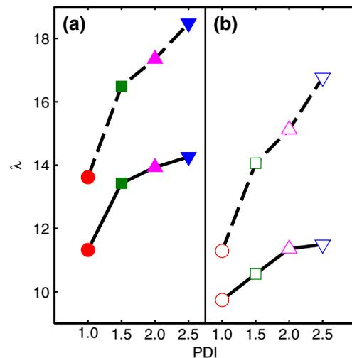
FIG. 2 (color online). Penetration depth,  $\lambda$  (in units of  $d$ ), of matrix chains into grafted layer on nanoparticles ( $D = 5d$ ) grafted with polydisperse chains with  $N_{g,\text{avg}} = 20$  at  $\sigma = 0.10$  chains/ $d^2$  (solid lines) and  $\sigma = 0.25$  chains/ $d^2$  (dashed lines) in a dense solution ( $\eta = 0.1$ ) of monodisperse homopolymer matrix chains with  $N_{\text{matrix}} = 10$  (filled symbols) and  $N_{\text{matrix}} = 40$  (open symbols).
