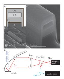
FIG. 1 (color). Experimental structure and measurement setup. (a) Schematic of the end facet of the n=0 waveguide showing the Si/Cr/Ag/SiO<sub>2</sub>/Ag/Cr multilayer structure. (b), (c) Scanning electron micrographs of a  $2-\mu$ m-long, focusedion-beam fabricated waveguide. (d) Setup for the angle- and spectrally resolved collection of light in the SEM chamber using a parabolic mirror placed over the sample.
