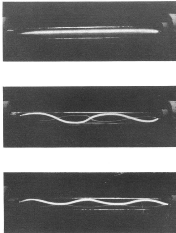
FIG. 2. Constricted krypton discharge.  $p = 23.5$  mm Hg,  $I = 40$  mA. Top: Unmodulated. Center: 90% modulation,  $\omega_{0,1}/2\pi = 5.56$  kc/sec. Bottom: 65% modulation,  $\omega_{1,0}/2\pi = 11.60$  kc/sec.
