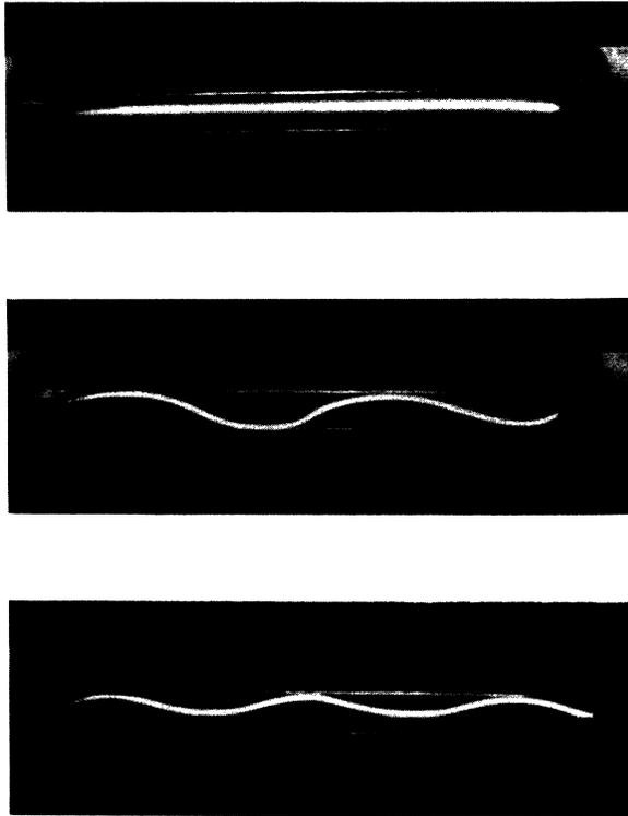
FIG. 2. Constricted krypton discharge.  $p = 23.5$  mm Hg,  $I = 40$  mA. Top: Unmodulated. Center: 90% modulation,  $\omega_{0,1}/2\pi = 5.56$  kc/sec. Bottom: 65% modulation,  $\omega_{1,0}/2\pi = 11.60$  kc/sec.
