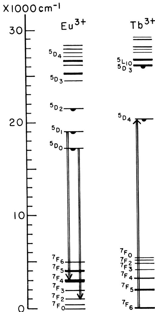
FIG. 2. Energy-level diagrams of the  $Tb^{3+}$  ion and the  $Eu^{3+}$  ion [following Thomas *et al.* (references 4 and 5)]. The excitation of the Tb and the fluorescence of the Eu in  $(Tb_{0.8}Eu_{0.2})_2(WO_4)_3$  in the present experiment are indicated by the arrows.
