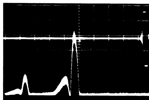
FIG. 2. Anomalous sound propagation under gain conditions in the same CdS crystal as used in Fig. 1. The main pulse has been amplified 20 dB over its dark level by application of an electric field of 1500 \text{ V/cm} . Pulse A: Anomalous trailing pulse. Pulse 3 and B: Echoes in quartz rod of pulses 1 and A.
