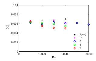
FIG. 3 (color online). Impact of viscosity variations on the time-averaged mean scalar dissipation rate  $\langle \epsilon \rangle$ . All simulations are for the analogue-fluid system with different values of log-viscosity ratio (R = -2 to 2). For each value of R, we plot  $\langle \epsilon \rangle$  as a function of Ra.
