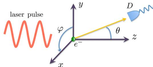
FIG. 1 (color online). Sketch of the system. The laser pulse impinges on the electron, initially located at the coordinate origin. The scattered radiation is observed on the detector  $D$ . The incoming pulse is linearly polarized along the  $y$  axis.
