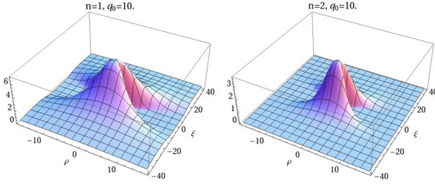
FIG. 4 (color online). The function  $\Gamma^{(n)}(q(\rho, \xi))$ , showing the region in space where the scattered radiation is produced, is plotted in two cases. For  $n > 1$ , photons are produced in the region where  $q \geq 1$ . The region where  $n = 1$  photons are scattered is larger since they are the only outcome of the non-relativistic regime  $q \ll 1$ .
