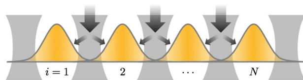
FIG. 1 (color online). Driven-dissipative chain of coupled cavities. Each cavity exhibits a large optical nonlinearity and sustains a single Wannier mode which weakly overlaps with its nearest neighbors, thus allowing for photon hopping between sites. Parametric pumps (depicted by arrows) couple to the weak intercavity field and inject photon pairs which, owing to strong photon-photon repulsion, split up into different cavities, effectively giving rise to  $p$ -wave pairing.
