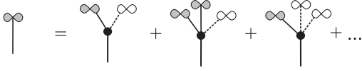
FIG. 4. Diagrammatic representation of Eq. (1) in a system of two interdependent networks a and b . The probability X_a , represented by a shaded infinity symbol, can be written recursively as a sum of second-neighbor probabilities. Open infinity symbols represent the equivalent probability X_b for network b , which obeys a similar recursive equation.
