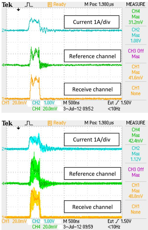
FIG. 6 (color online). Experimental results: the collector current and the detector’s voltage readings in the two channels are seen. (a) A single typical pulse. (b) The accumulation of many subsequent pulses.
