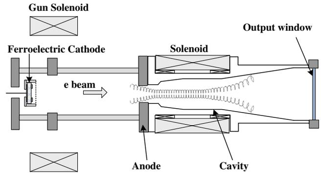
FIG. 3 (color online). The experimental setup of the ferroelectric cathode 95 GHz gyrotron.
