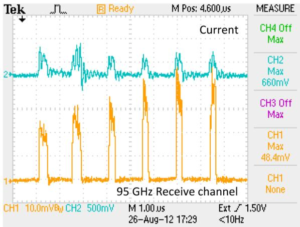
FIG. 8 (color online). Operation at  $\sim 0.7$  MHz repetition rate,  $\sim 25\%$  duty cycle, and above 1 kW average power during a macropulse of the solenoid.
