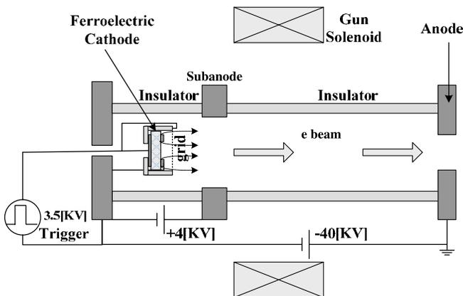
FIG. 2 (color online). The ferroelectric electron gun arrangement.
