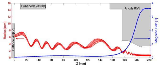
FIG. 4 (color online). Simulation of the electron beam trajectory.
