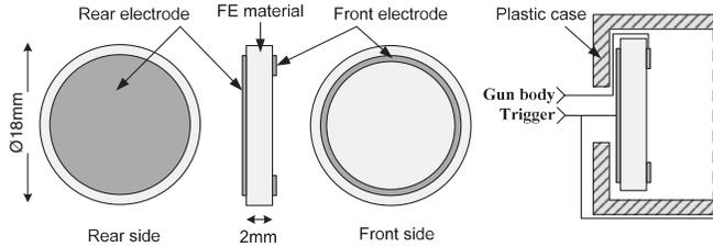
FIG. 1. The ferroelectric (FE) cathode arrangement.
