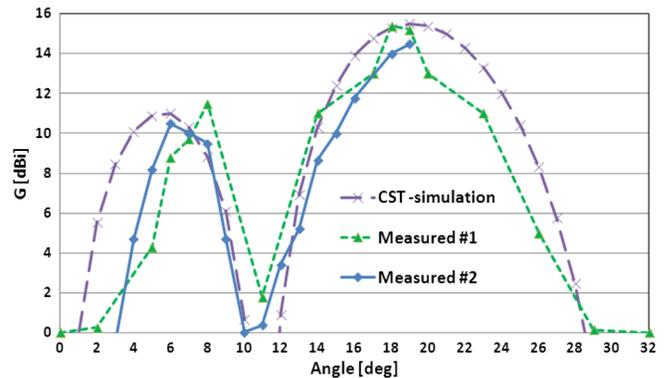
FIG. 7 (color online). Measurement and theoretical evaluation of the radiated pattern.
